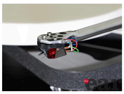
The other benefit of the Nd housing is that the bolts thread into the top of the cartridge and there is no need to screw small nuts onto tiny bolts. The holes in the Nd3 do not have brass inserts for the bolts to screw into but a thread is cut into the body. Given that the body is plastic I was concerned that tightening with the Rega torque driver might strip the thread but was assured that this is the way they are fixed in the factory. It must be decent plastic.
