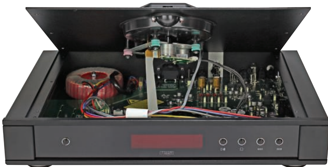
This top loader uses Wolfson WM8472 digital converter (DAC) chips and is driven by a linear power supply fed by a toroidal transformer (left rear).
