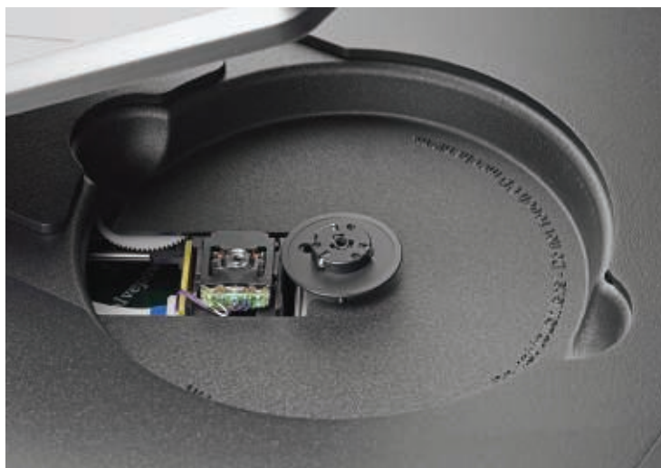
The transport holds a CD in place on the spindle-hub with three spring-loaded clips. Also seen here is the sled holding the upward firing laser that moves from centre outward.
